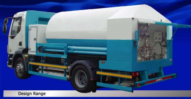
The Carrymore<sup>™</sup> range offers the air gas industry a wide choice of micro-bulk units in capacities from 2000 to 17000 litres and working pressures from 2 to 22 bar with optimised units for nitrogen, oxygen, argon and Co2
