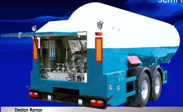
The Stainless Steel Carrymore range offers the air gas industry market leading payloads in capacities from 17000 to 60000 litres with optimised designs for oxygen, argon and nitrogen as well as more specialised units for ethylene, nitrous oxide and L.N.G.
